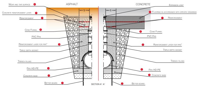
The best condition for an easy installation of the FUNNEL is that the slope of the pipe and the slope of the finished paving are the same.
